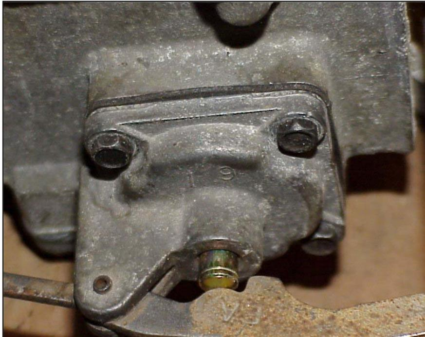
Insert the accelerator pump rod into the proper hole on the pump arm. Attach the other end of the rod to the throttle with the retainer into the third hole.
