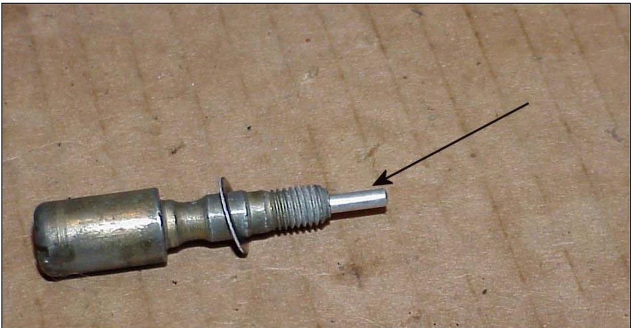
Now very carefully insert the hollow screw into the venturi cluster. You can also insert the weight into the hole first than the hollow screw. You may have to shake things a little to get the screw to drop over the rod.
