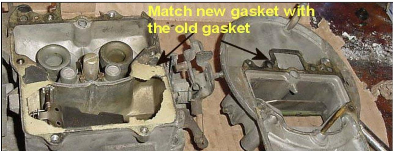
Remove the carb internals starting with the float. The rod that holds the float is secured by the wire clip that runs behind the needle seat. Use a pair of long nose pliers to remove the wire clip and the rod with the float can then be removed.
