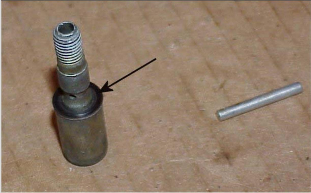
Insert the weight into the hollow screw.
