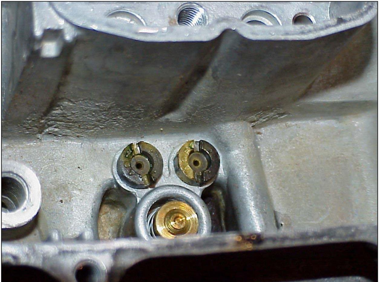
Next put the needle seat in. There should be a gasket between the needle seat and the carb.
