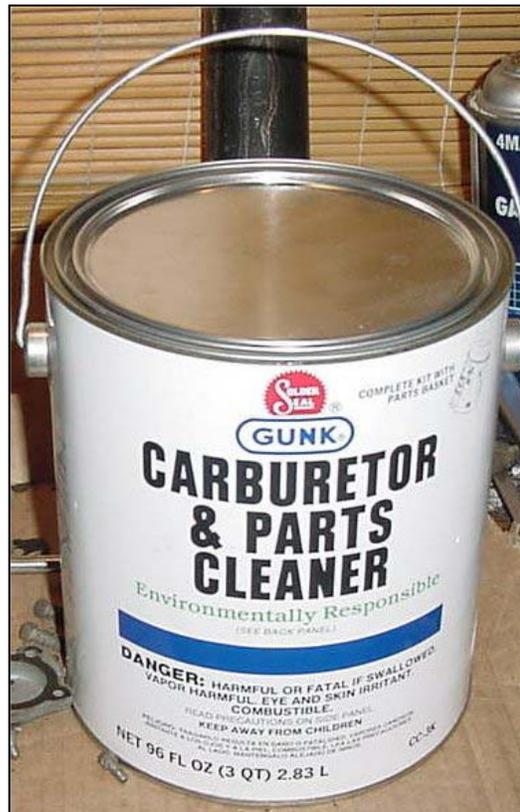
**All plastic pieces, choke, float, pull off valve, power valve, and gaskets should not be soaked.**
