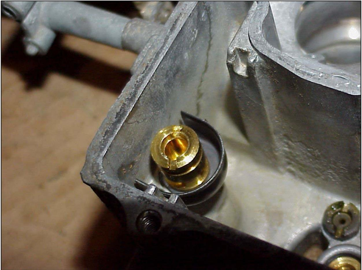
Install the float clip onto the needle.
