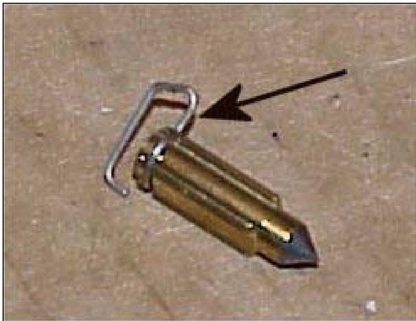
Put the needle in the needle seat. In this case I did not remove the old retaining rod. If you want to replace it, slide the float over the rod and then attach the wire retainer to the rod. The wire retainer sits in grooves in the rod.
